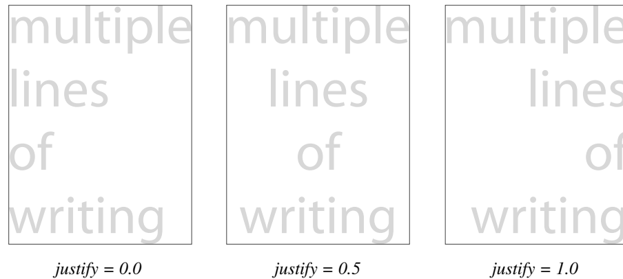
Figure A.6 The justify parameter controls the horizontal positioning of multiline text within the bounding box.
